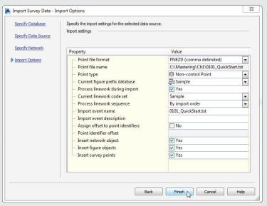
See the sections "The Figure Prefix Database" and "The Linework Code Set Database" in Chapter 2 for more information on creating figures and importing survey data.
