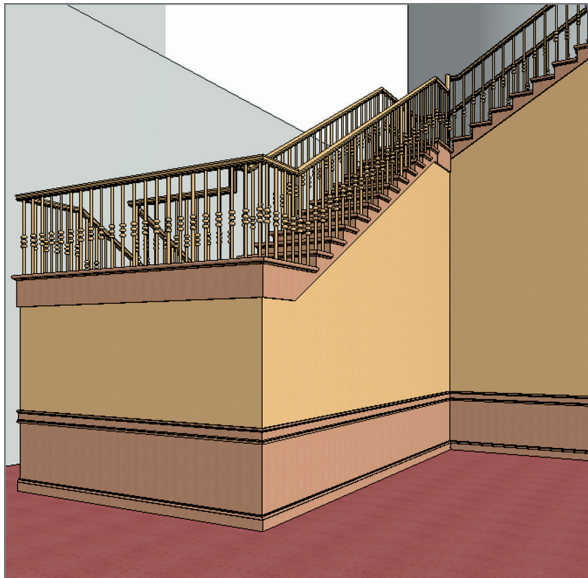
FIGURE BC1.15: The finished walls should follow the profile of the stairs.
