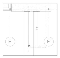
FIGURE 10.82: Pick the first point on the landing, and then move your cursor down 15'-0'' (4500 mm).
