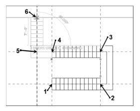
FIGURE 10.63: Picking the intersections of the reference planes to determine where the stairs will go
