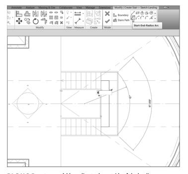
FIGURE 10.7: Add a radius to the outside of the landing.
