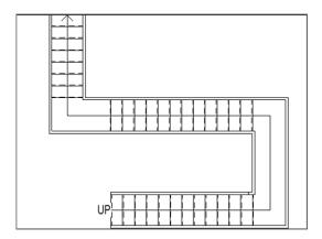
FIGURE 10.65: The stairs as shown in plan
