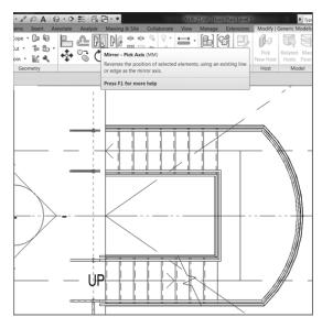
FIGURE 10.25: Mirroring and configuring the two railing extensions
