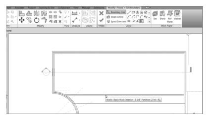
FIGURE 10.54: Adding the floor outline to the walls. Be sure to offset the line 5'-0'' (1500 mm) from the south wall. This will be the stair landing.
