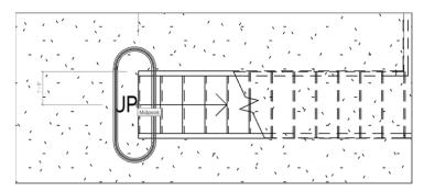
FIGURE 10.67: Placing the landing
