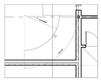
FIGURE 10.36: Picking the third point to form the arc. It will be tangent upon the first two points you picked.
