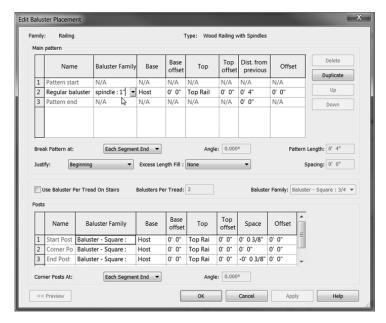
FIGURE 10.57: Adding the spindle to the Main Pattern area
