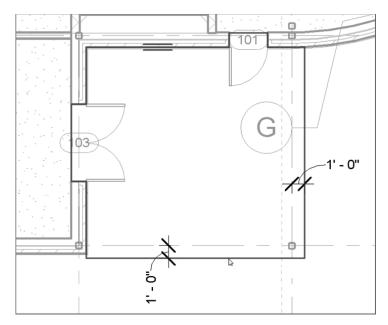
FIGURE 10.79: Sketching the slab perimeter
