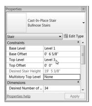
FIGURE 10.61: The Base Offset value is set to 65/8" (152 mm).
