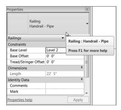
FIGURE 10.49: Setting the landing handrail type
