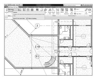
FIGURE 10.45: Adding the perspective view
