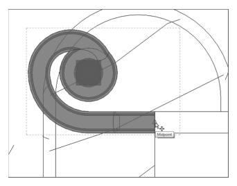
FIGURE 10.70: Moving the post to align with the stair railing
