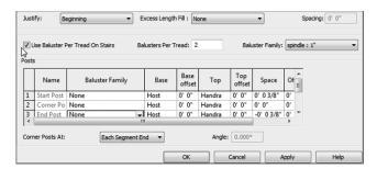
FIGURE 10.58: Specifying two balusters per tread and no actual posts
