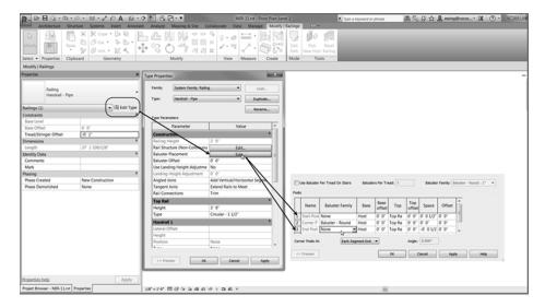
FIGURE 10.23: Configuring the default settings for the railing type Handrail - Pipe - Horizontal Railing
