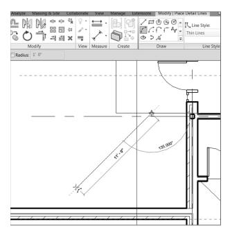
FIGURE 10.35: With the Start-End-Radius Arc button selected, start at the midpoint of the landing and then go southwest at an angle of  $135^{\circ}$  and a distance of 11'-0'' (3300 mm).
