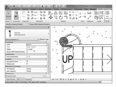
FIGURE 10.69: Placing the post with the gooseneck
