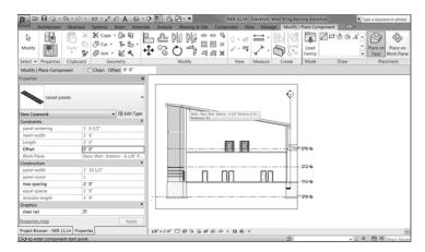
FIGURE 10.75: Picking the far wall to establish a work plane
