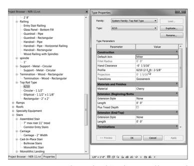
FIGURE 10.56: Changing the rail. Note that you can add as many rails as you want. Here, you're adding only one.
