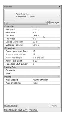
FIGURE 10.3: Changing the Element Properties of the stairs
