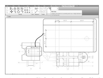
FIGURE 10.62: Using dimensions to lay out the centerlines of the stairs
