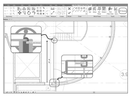
FIGURE 10.24: Sketching the path of the railing
