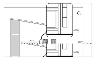
FIGURE 10.76: Adding the line-based, raised-panel family
