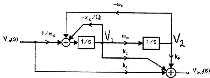
$$V_1 = \frac{1}{s} \left[ \frac{1}{\omega_0} V_{in} - \omega_0 V_2 - \frac{\omega_0}{Q} V_1 \right] \quad (1)$$
