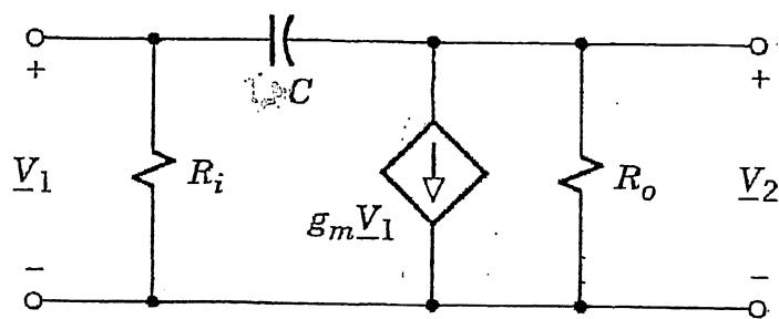
2. The two-ports shown have same impedance matrices. Find the impedance  $Z_x$ .
