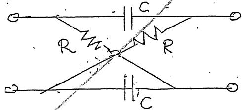
2. a. Find the chain matrix  $T$  of a gyrator with gyration resistance  $R$ .
