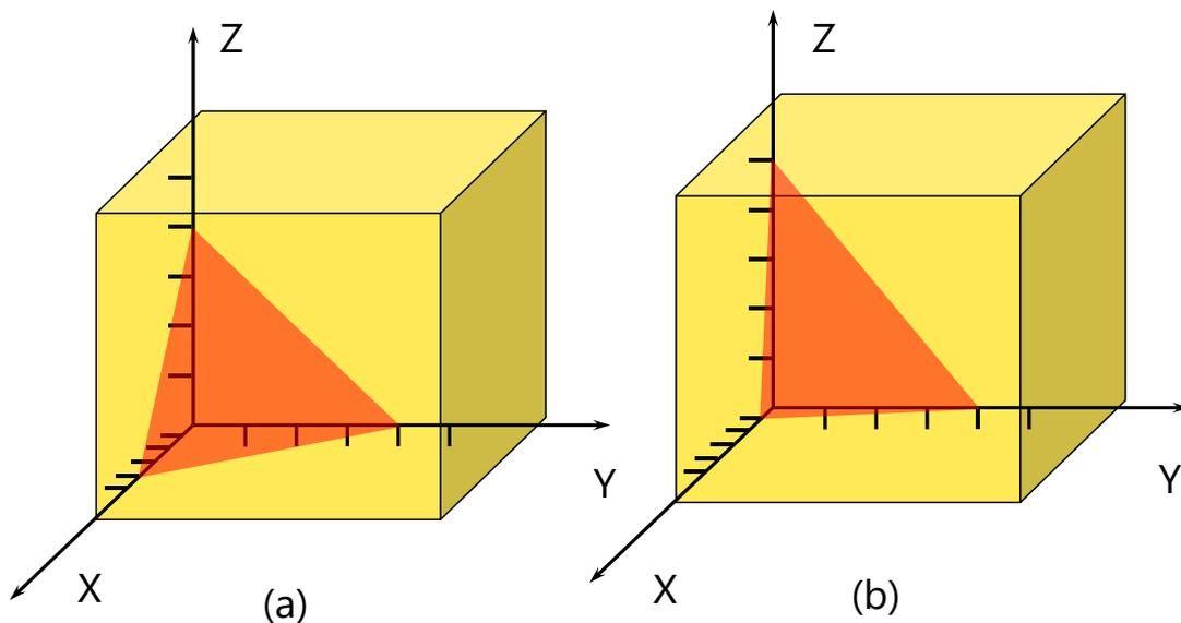
**Figure 2:** Cubic crystal structures with two different crystal planes located. The tick marks are evenly spaced.
