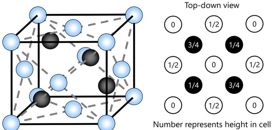
**Figure 1:** Diamond crystal structure (crystal structure of germanium). All atoms are silicon, despite the differences in color. The difference in color is intended to make the cell easier to visualize.
