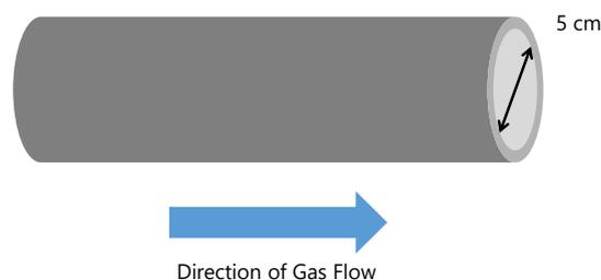
**Figure 4:** Schematic diagram of pipe through-which  $\text{N}_2$  gas is flowing. The internal diameter of the pipe is 5 cm.
