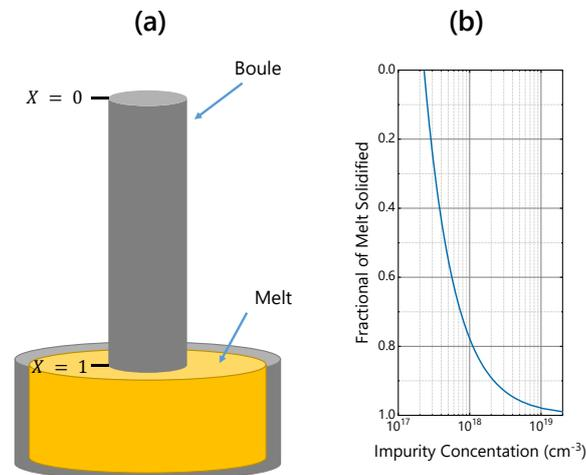
**Figure 3:** (a) Schematic diagram of boule of silicon withdrawn from melt. (b) Impurity concentration in the silicon boule as a function of the fraction of the melt that has been solidified. This data can be downloaded [here](#).
