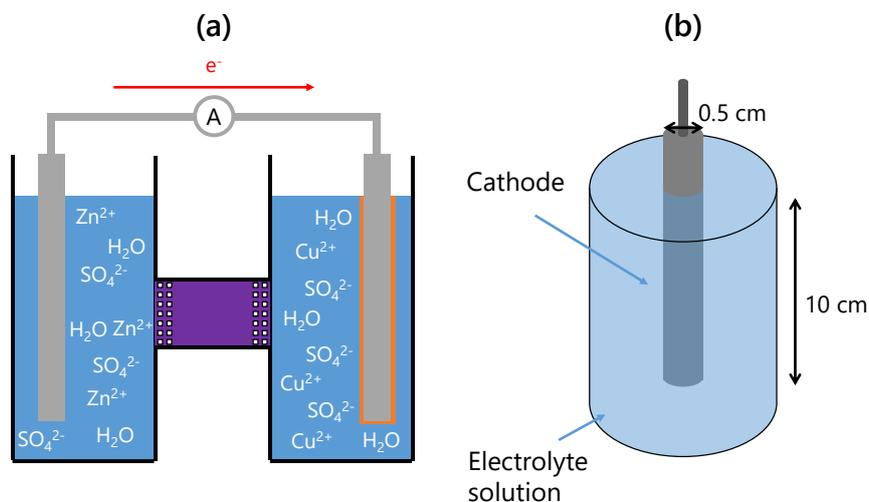
**Figure 5:** (a) Schematic diagram (side view) of simple galvanic cell. Electrons flow from the anode in electrolyte solution 1 on the left to the cathode in electrolyte solution 2 on the right. The purple region in the middle of the cell is the salt bridge. (b) An oblique view of the cathode in solution 2. The cathode is cylindrical, has a diameter of 0.5 cm and a submerged length of 10 cm.
