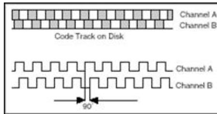
Figure 2. Quadrature Encoder A and B Output Signals
