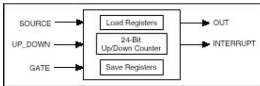
Figure 3. Simplified Model of a Counter
