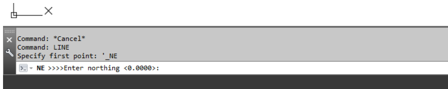
FIGURE 1.9 A view of the command line while a transparent command (covered later in this chapter) is used to draw a line. Notice how the command line reports that the LINE command has been started and then prompts for the first piece of information: the “first point.”
