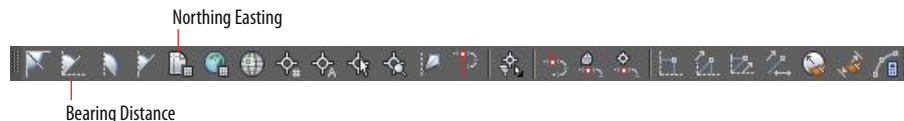
FIGURE 1.11 The Transparent Commands toolbar with red lines pointing to the Bearing Distance and Northing Easting transparent commands
