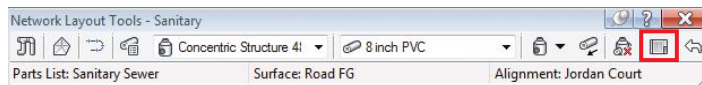
FIGURE 14.15 The Pipe Network Vistas button highlighted on the Network Layout Tools toolbar
