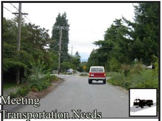
Traffic mobility and parking needs on NW 110th St. were not compromised by the addition of wide strips of vegetated swales. A round traffic circle at the intersection of 1st Ave. NW and 110th St. helps to calm traffic. While more space is devoted to drainage and less to pavement, two large vehicles, such as fire trucks or delivery trucks, can easily pass each other.
