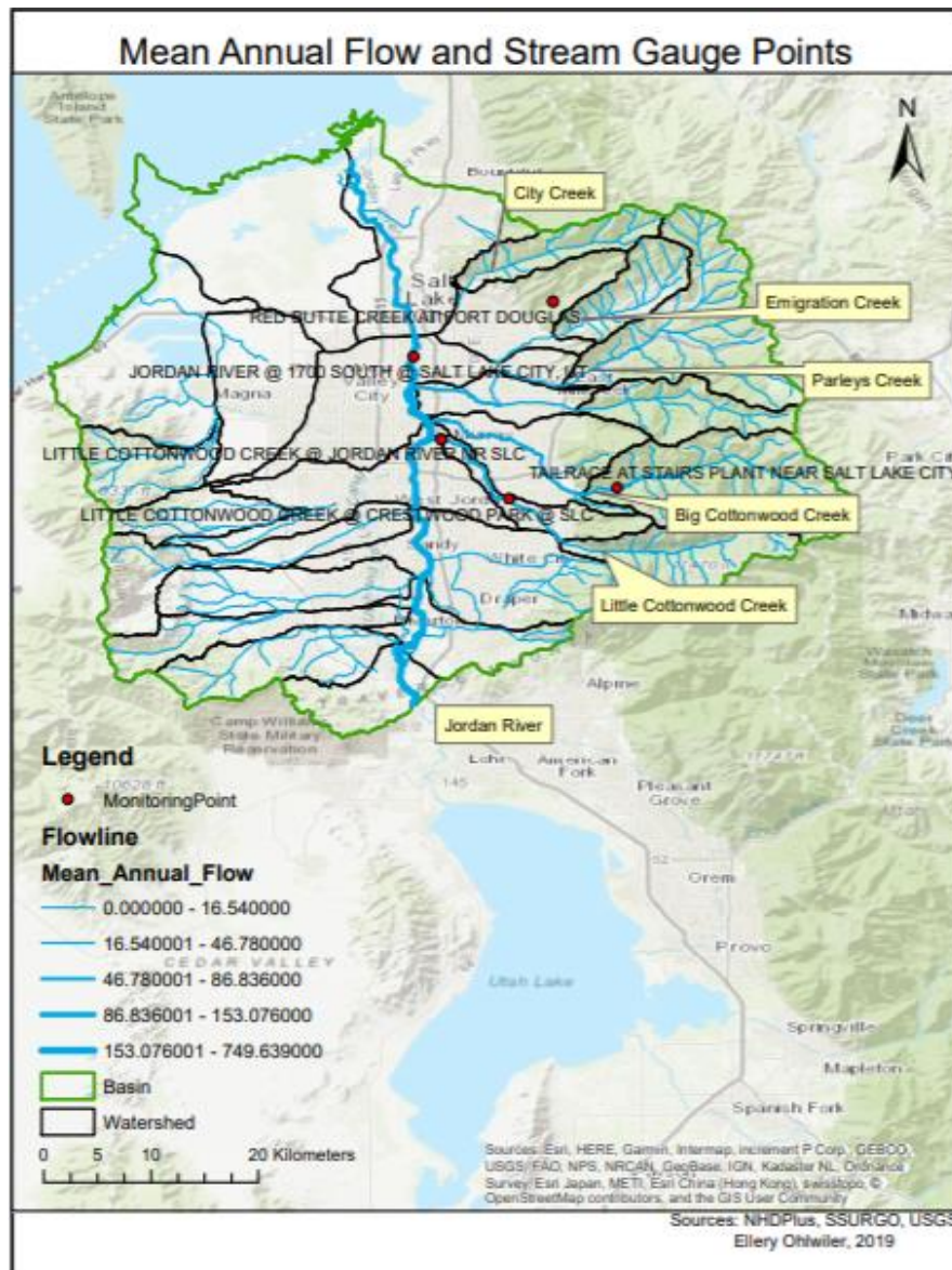
Figure 11. Flowline map for mean annual flow with major streams and monitoring points
