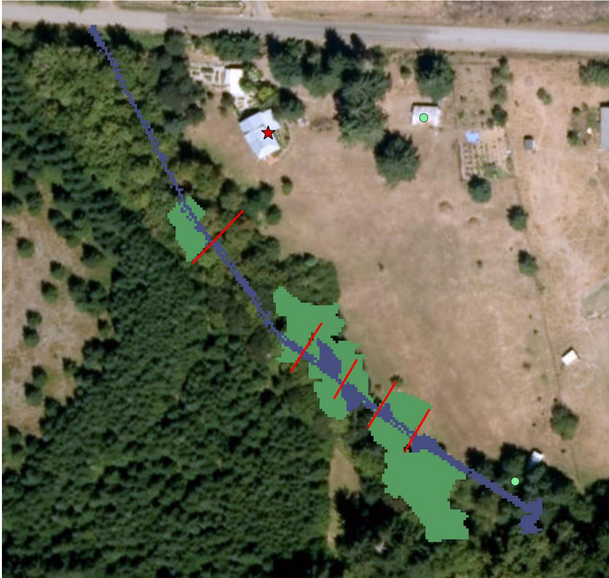
Figure 7. Estimated Flooded Area Without (purple) and With (green) BDAs on the Landscape at 3ft floodstage
