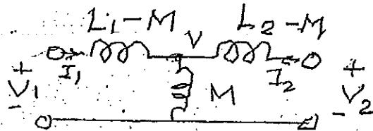
$$\boxed{T = [A \ B \ C \ D]} = \boxed{\begin{bmatrix} z_{11}/z_{21} & |z_1|/z_{21} \\ 1/z_{21} & z_{22}/z_{21} \end{bmatrix}} = \boxed{\begin{bmatrix} L_1/M & s(L_1 L_2 - M^2)/M \\ 1/sM & L_2/M \end{bmatrix}}$$
