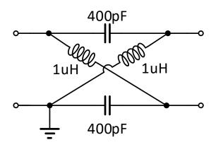
2. Find the short-circuit admittance matrix of the bridged-T two-port at f = 1MHz.
