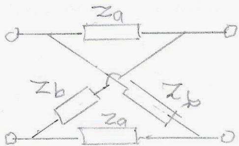
2. The two two-ports shown below are equivalent. Find the element values of the ladder circuit.
