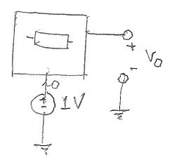
1. Find the output voltage of the circuit shown using interreciprocity. All impedances are equal.
