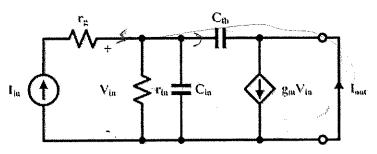
$$\omega_r^2 = \left[\frac{q_{ab}^2 - 1/r_{in}^2}{C_{in}^2 + 2C_{in}C_{fb}}\right]$$
