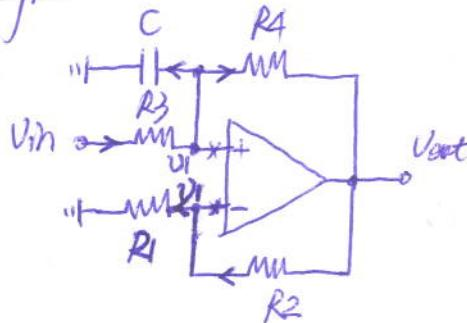
$$\Rightarrow H(s) = \frac{V_{out}}{V_{in}} = \frac{(G_1 + G_2)G_3}{sG_2C + G_2G_3 - G_1G_4}, \quad G_i = \frac{1}{R_i} \quad (i=1,2,3,4)$$
