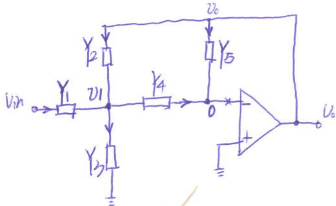
$$\Rightarrow H(s) = \frac{V_{out}}{V_{in}} = - \frac{Y_1 Y_4}{Y_1 Y_5 + Y_2 Y_4 + Y_2 Y_5 + Y_3 Y_5 + Y_4 Y_5}$$
