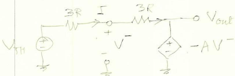
$$I = \frac{V_{Th} - V_{out}}{6R} = \frac{1}{3R} \left( -\frac{1}{A} - 1 \right) V_{out} = -\frac{\mu+1}{3R} V_{out}$$
