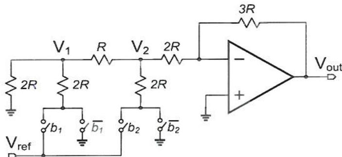
2. a. Find the STF and NTF of the  $\Delta\Sigma$  ADC shown. Use  $H(z) = z^{-1}/(1-z^{-1})$ .
