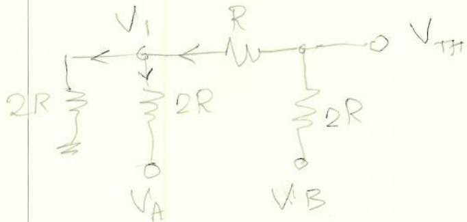
$$\frac{V_1}{2R} + \frac{V_1 - V_A}{2R} = \frac{V_B - V_1}{3R}$$
