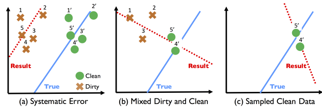
Figure 1: (a) Systematic corruption in one variable can lead to a shifted model. The dirty examples are labeled 1-5 and the cleaned examples are labeled 1'-5'. (b) Mixed dirty and clean data results in a less accurate model than no cleaning. (c) Small samples of only clean data can result in similarly issues.
