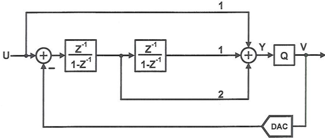
3. The circuit of the  $\Delta\Sigma$  modulator MODA shown in Fig. A is redesigned as illustrated in Fig. B, to allow more time for quantization. The integrator transfer function is  $I = 1/(z - 1)$ .
