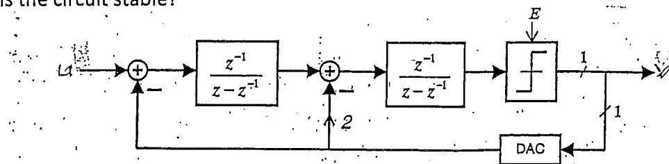
3. In the  $\Delta\Sigma$  ADC shown,  $I(z) = 1/(z - 1)$ . Two-bit quantization is used, and  $V_{ref} = 3$  V.
