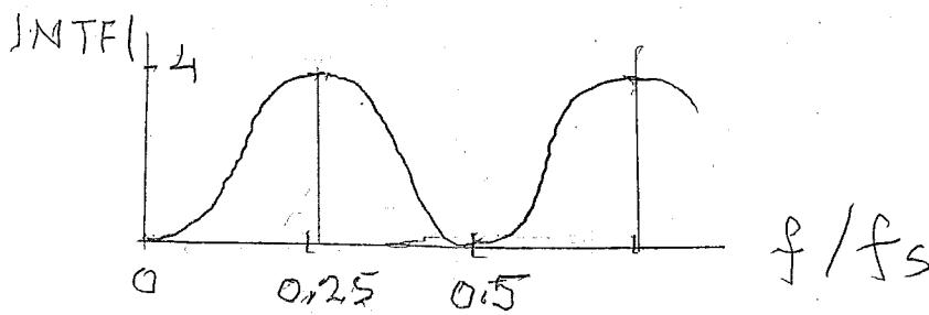
c. The NTF is that of MOD2, with  $z$  replaced by  $z^2$ , same for STF. So both frequency responses are compressed by 2, and the time responses stretched by 2. Since MOD2 is stable, so is this system, for a range of inputs.
