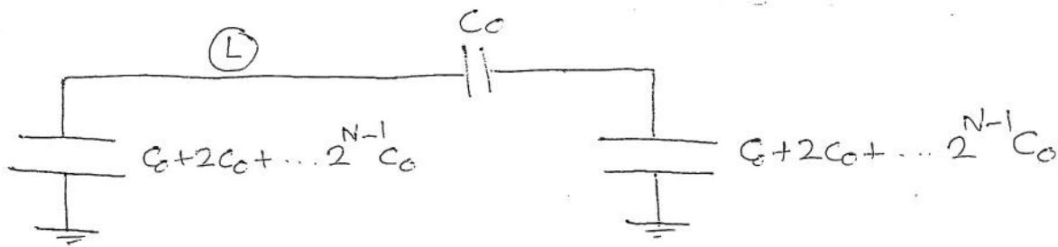
$$\text{Now } C_0 + 2C_0 + \dots + 2^{N-1}C_0 = (2^N - 1)C_0$$
