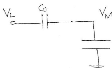
$$V_M = V_L \times \frac{C_0}{C_0 + (Q-1)C_0}$$
