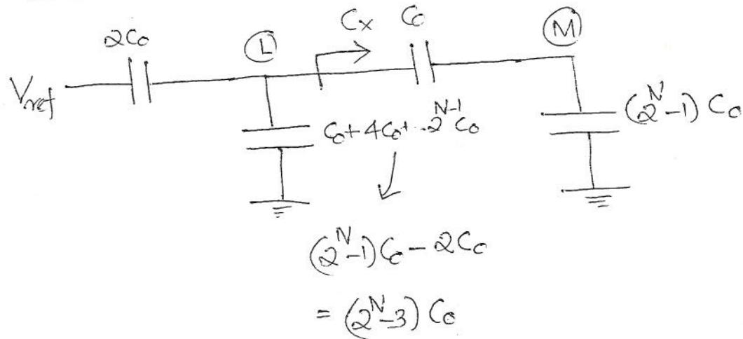
$$V_L = \frac{2C_0}{2C_0 + C_x + (2^N - 3)C_0} \cdot V_{ref} = V_{ref} \times \frac{2C_0}{(Q-1)C_0 + C_x}$$
