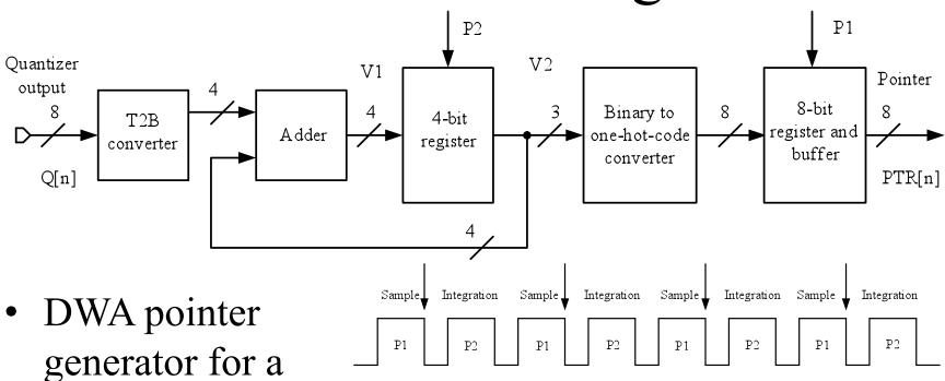
DWA pointer generator for a 9-level quantizer with barrel shifter
