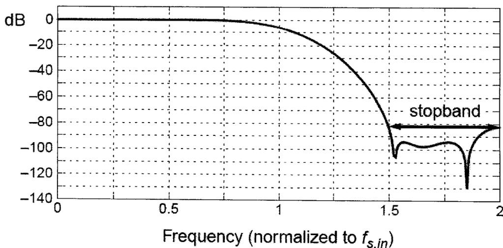
82 dB image attenuation. It requires 44 additions, 50 registers. Halfband filter (symmetric response, fewer tap weights).
