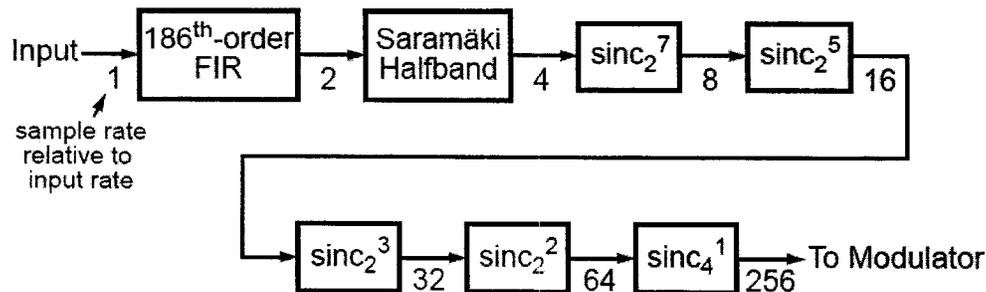
Here, the  $\text{sinc}_N^k$  filter has the transfer function
