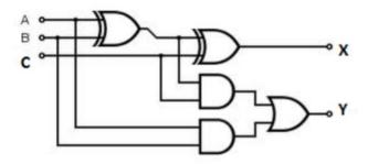
It's just a full adder. Inputs A and B are corresponding bits of two binary numbers that are to be added. Input C is "carry in". Output X is the sum bit, and output Y is the "carry out" bit.
